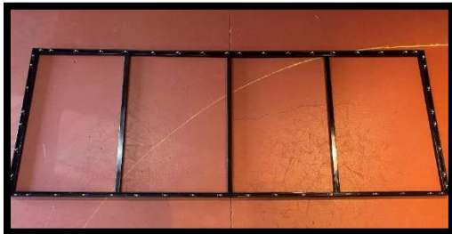
Face can be assembled piece by piece on the posts or pre-assembled as shown.
